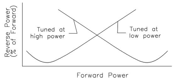
FIGURE 4 – Reverse power as percentage of forward power for tuned high Q load.
