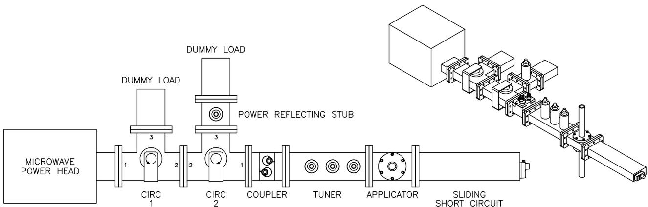
FIGURE 5 – Waveguide Configuration for variable microwave power at constant frequency.
