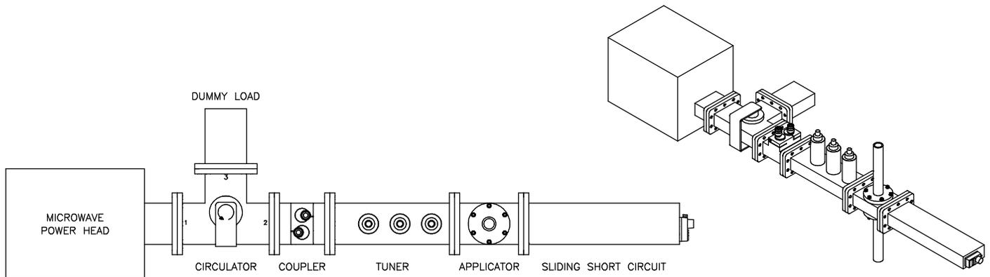
FIGURE 3 – Typical waveguide configuration for microwave heating.
