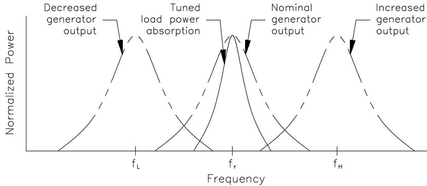
FIGURE 2 – Output frequency shifting with changes in output power.
